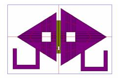
In first design bandwidth was not sufficiently large so stubs of length 150 mm and width 10 mm are attached with triangular shape at the center on a side of triangle. Through this bandwidth of antenna is widened but size of antenna was not comfortable for practical use.
